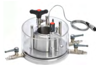
KO CONSOLIDATION CELL for measuring radial stress
