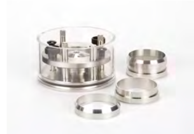
COMBINED FIXED & FLOATING RING CELL
