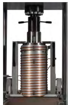
High pressure /High temperature Triaxial cell with external cooling system
